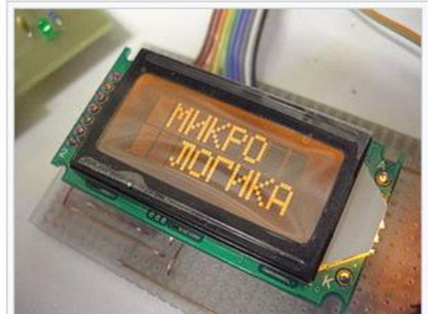
Amber backlight on a HD44780 display
